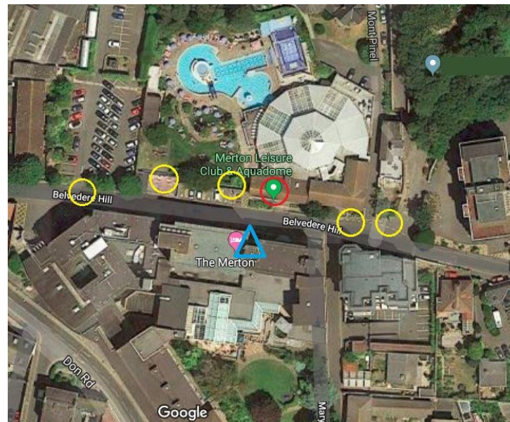
Figure 3- Survey Area with Spot Measurement Markers: The blue triangle is the site location, the yellow circles are intermediate locations measured at during the peak search and the red circle is the spot where the highest spot search reading was obtained and where the detailed survey was carried out
