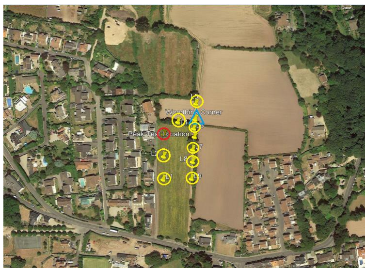
Figure 3- Survey Area with Spot Measurement Markers: The blue triangle is the site location, the yellow circles are intermediate locations measured at during the peak search and the red circle is the spot where the highest spot search reading was obtained and where the detailed survey was carried out
