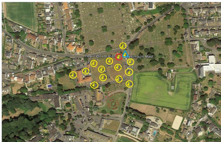
Figure 3- Survey Area with Spot Measurement Markers: The blue triangle is the site location, the yellow circles are intermediate locations measured at during the peak search and the red circle is the spot where the highest spot search reading was obtained and where the detailed survey was carried out
