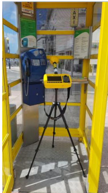
Figure 3- The probe was positioned inside the kiosk where the strongest signal was recorded
