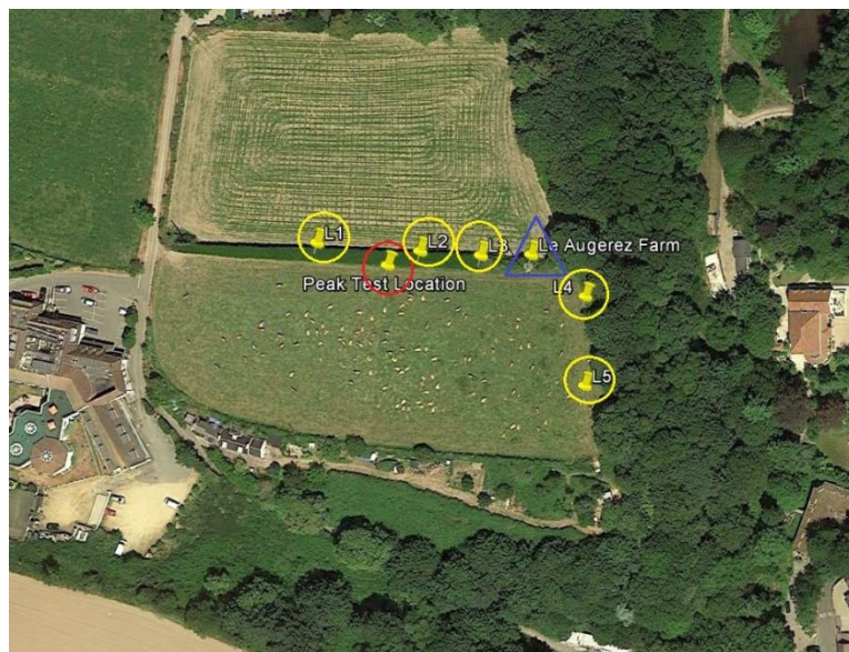
Figure 3- Survey Area with Spot Measurement Markers: The blue triangle is the site location, the yellow circles are intermediate locations measured at during the peak search and the red circle is the spot where the highest spot search reading was obtained and where the detailed survey was carried out
