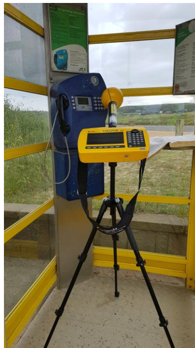
Figure 3- The probe was positioned inside the kiosk where the strongest signal was recorded
