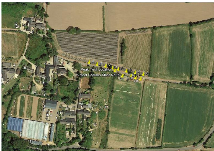
Figure 3- Survey Area with Spot Measurement Markers: The blue triangle is the site location, the yellow circles are intermediate locations measured at during the peak search and the red circle is the spot where the highest spot search reading was obtained and where the detailed survey was carried out
